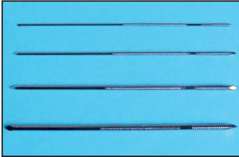
Fig 4. The Miniature IMEX Interface Fixation Half-Pins are threaded Kirschner wires with trocar points on both the smooth and threaded ends. The central area of the pin shank is roughened to improve the interface with methymethacrylate, which is often used in conjunction with this system.
