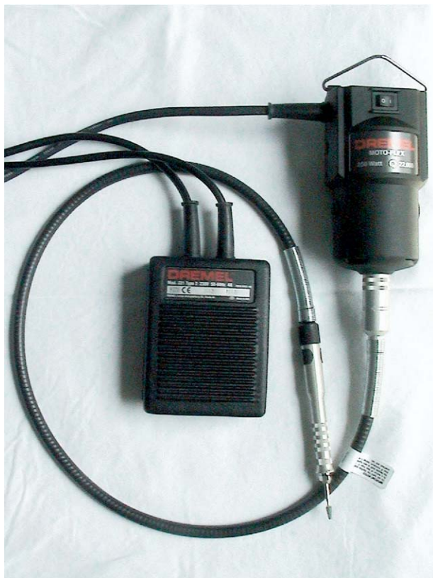
Figure 14. Heavy-duty flex shaft Dremel with straight handpiece and foot lever for speed control (Reprinted from Capello V, et al: Rabbit and Rodent Dentistry Handbook, 2005, with permission from Zoological Education Network, Lake Worth, FL).
